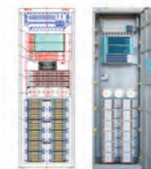
Schematic diagram of indoor jumperless cross connection cabinet for optical cable (integral structure diagram)
