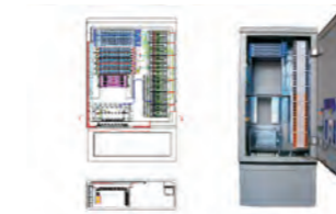
Schematic diagram of outdoor jumperless cross connection cabinet for optical cable (integral structure diagram)
