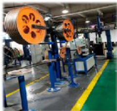
Equipment automation transformation, automatic mechanical winding arrangement, production personnel decreased from 32 to 24.
